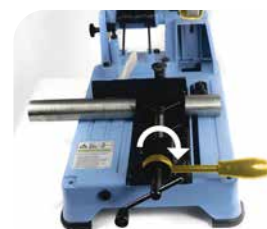
5. Turn the lever to the right and start the sawing process: next steps: 3 - 4 - 5.
