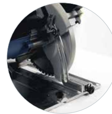
Depth adjustment with scaling
