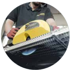
Ideal for cutting metal sheets, gratings and sandwich panels up to 67 mm
