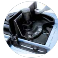
MITER CUTS CAN BE ADJUSTED WITHOUT TOOLS 90-75-60-45°
